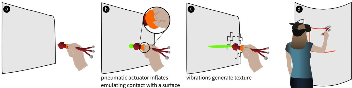
**Figure 1:** (a) VRSketchPen recreates the feeling of (b) contact pressure and (c) textures of surfaces, which allows users to have a more realistic experience when (d) drawing in VR. VRSketchPen also uses the unconstrained haptic feedback interaction technique, that allows users to draw in both flat and curved surfaces without snapping the stroke to a virtual canvas.
