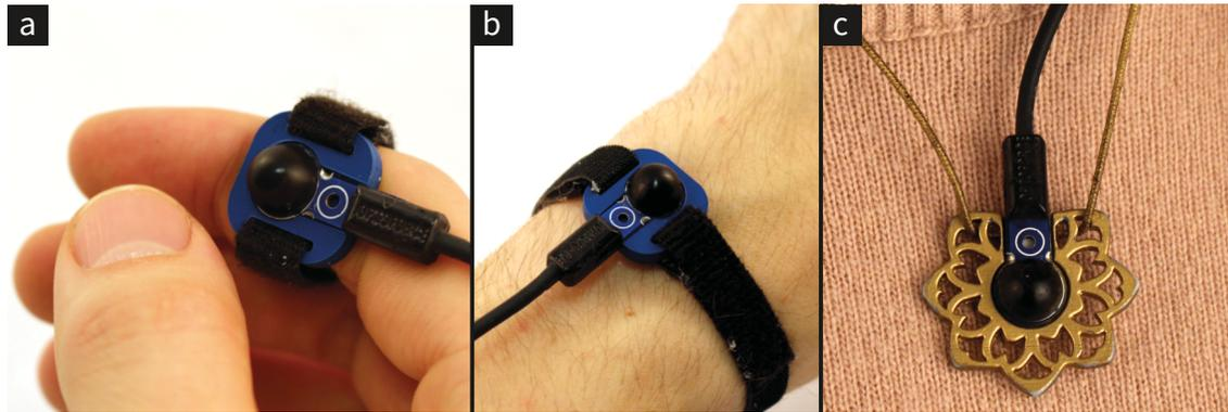
Fig. 2. Functional DeformWear prototypes: (a) ring, (b) bracelet, and (c) decorative pendant.
