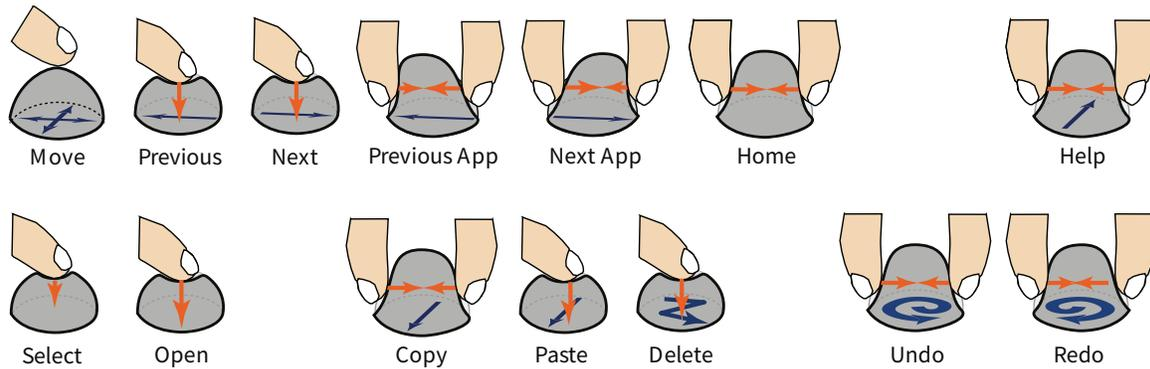
Fig. 7. Gestures for smartwatch interactions. Pressure and pinch forces are drawn in orange; shear forces in blue.
