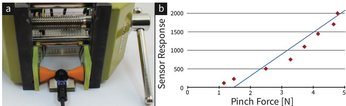
Fig. 6. Evaluation of pinch deformations: (a) apparatus; (b) sensor response for pinch forces with a fitted linear mapping function.
