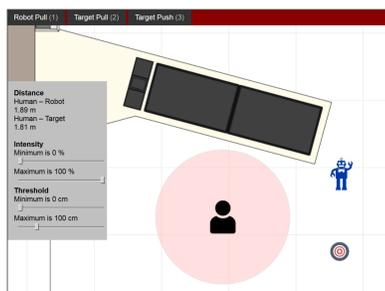
To control the belt we created a GUI. It allows a user to change the 2D positions of multiple entities (e.g., human and robot). The tactile stimulus is generated by a set of adjustable stimulus parameters and the relative arrangement of the entities.
