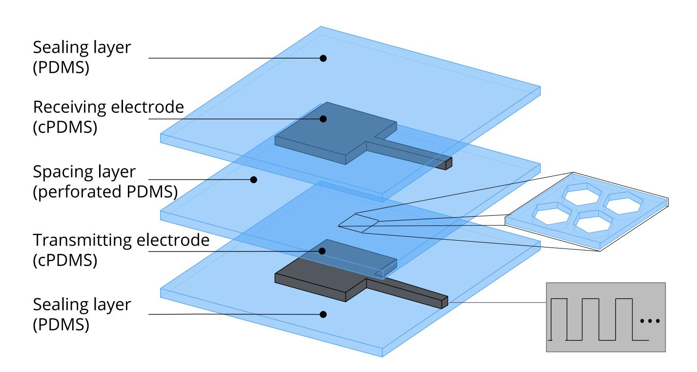
The sensor is a sandwich composed of multiple layers of silicone. Non-conductive parts are made of transparent PDMS, while conductors are realized with carbon-doped PDMS. Both materials are biocompatible, flexible and stretchable.
