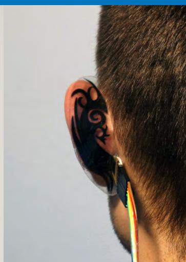
iSkin is a novel class of skin-worn sensors for touch input on the body. The sensor is a very thin overlay, made of biocompatible materials, and is flexible and stretchable. It can be produced in different shapes and sizes to suit various locations on the body.
