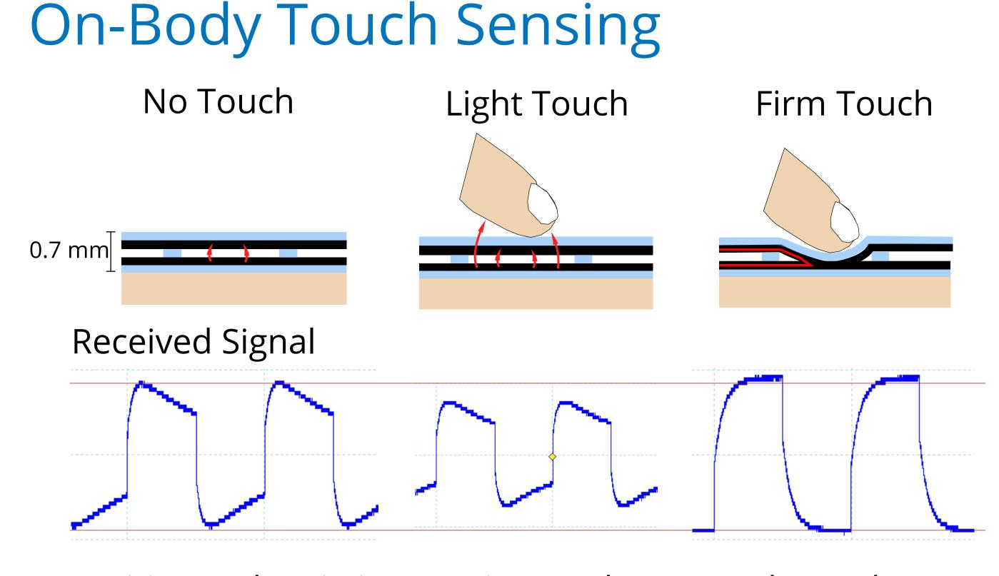
Capacitive and resistive sensing on the same electrode structure senses multi-touch, give precise real-time data about touch down and touch up, and can distinguish two levels of normal force.
